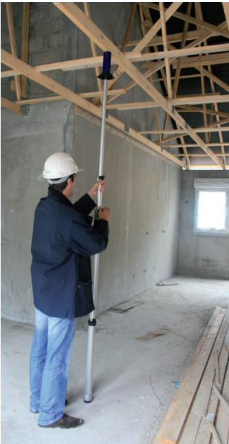
Measure heights up to 13' 4" (4 m) in tape measure mode.
